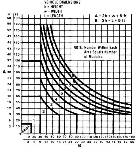
NOTE: This chart is normally reliable for vehicles of regular configuration. Vehicles of irregular configuration such as artillery pieces or cranes may require additional modules.
