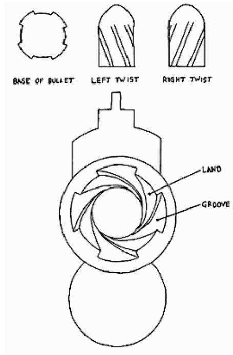
Bullets do not typically follow a straight line to the target. Rotational forces are in effect that keep the bullet off a straight axis of flight. These rotational effects are diagrammed below:
