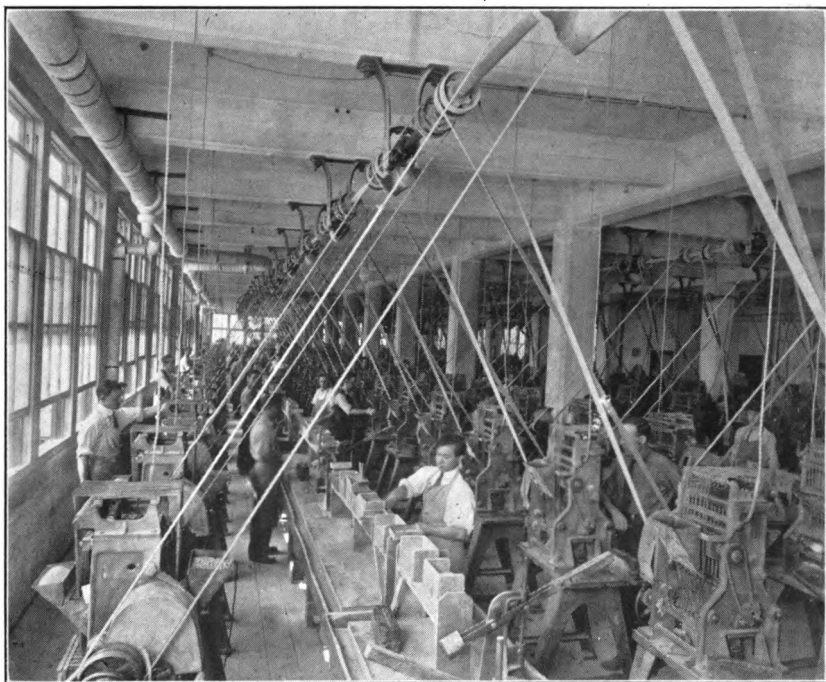
Loading 630 layers, alternately nickel hydrate and nickel flake, into a tube 4\frac{1}{2} inches long. See magnified section of tube above.
