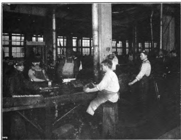
Loading the Negative Pocket with Iron Oxide.
