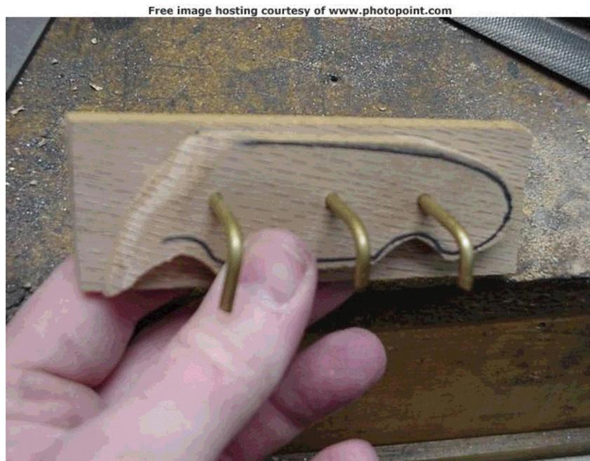
Check to see if left slab is good and flat and flush to the metal. If you need to, flatten on sand paper and the Kitchen counter top. Formica is usually pretty flat
