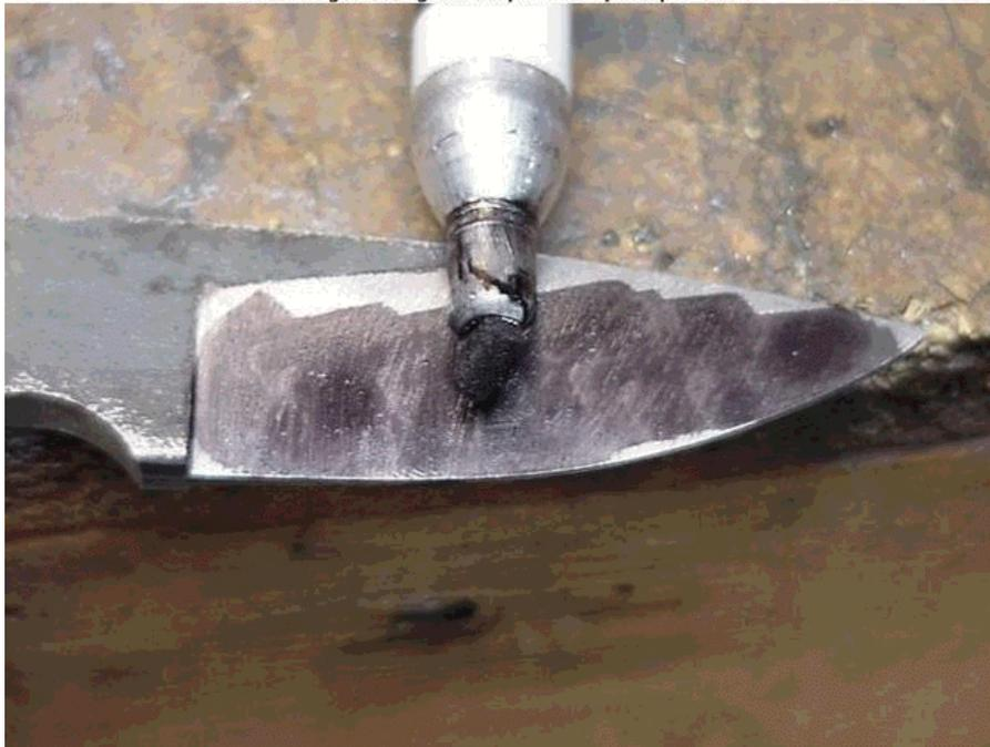
Trying to keep with the cheapo theme here is our sanding block, A paint stir stick. I first sanded along the area that would be called the plunge. I used the stir stick and 120 grit to clean this area up. Then I started sanding lengthwise plunge to tip until all the rough file marks are gone. This will also make it flat. Use a little soap and water as a lube to keep your sandpaper from loading up. Be sure to wipe the blade down dry when your done or you will have rust tomorrow.
