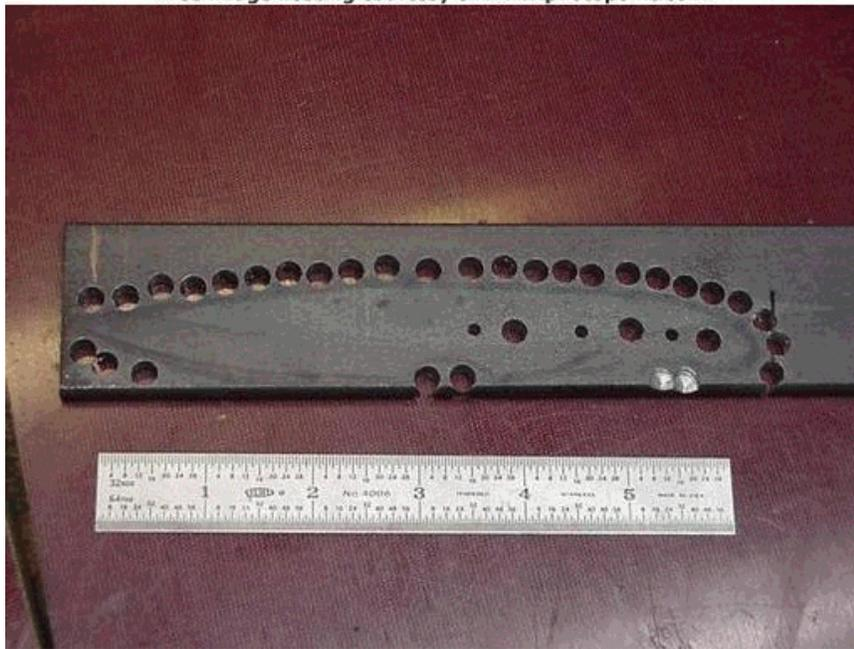
pic #2 Screw the blade to a bench or stump or whatever you have and cut out the handle portion only. Remove the material so you can file the handle to shape. Do this first because you won't have any way to screw the blade to the bench if you cut out the entire blade. do the handle work first! Once the handle is to a pretty good shape remove and screw to the bench through the handle and cut out blade.
