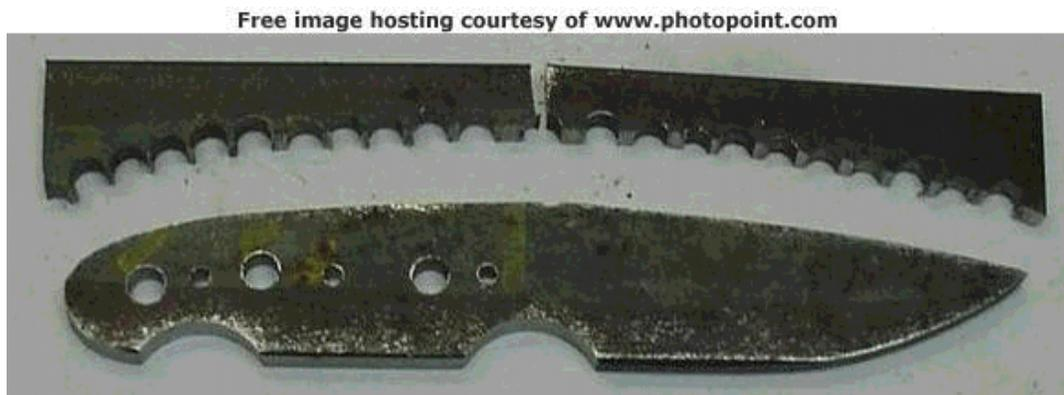
I marked the edge of the blade using my 1/4 inch drill bit. Black the edge using a marker or a sharpie. Slide the drill bit point along the edge and it will scribe a line. Turn the blade over and do the other side. You will get two lines about .025 to .030 apart. If the lines are two close re-black and roll the drill bit to move the point up or down accordingly and re-scribe. The lines will be about 1/2 the thickness of a penny apart.
