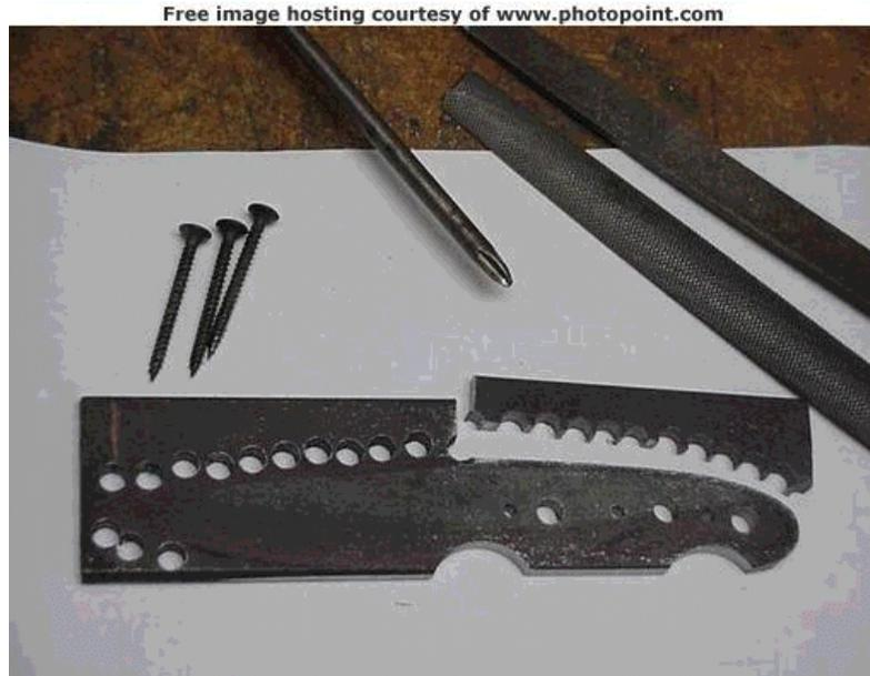
Ok , now I have the knife blank cut out and the edges filed. It is starting to take shape.
