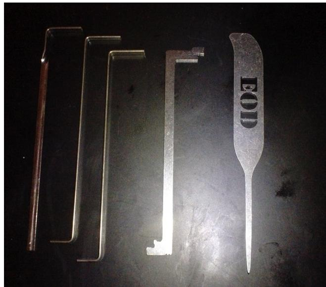
The selection of picks is heavy on raking tools as it is generally the fastest method of picking a lock. The kit also has a shank (marked with “EOD”) for bypassing locks with an exposed prawl.
