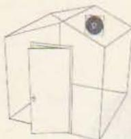
unless all of the surrounding door opening was blocked up – it was easier for the air to just pull in from the doorway around the fan rather than from the doorway clear across the greenhouse. Smarter folk put fans in the end wall above the door and kept it closed while opening the opposite door. In my
